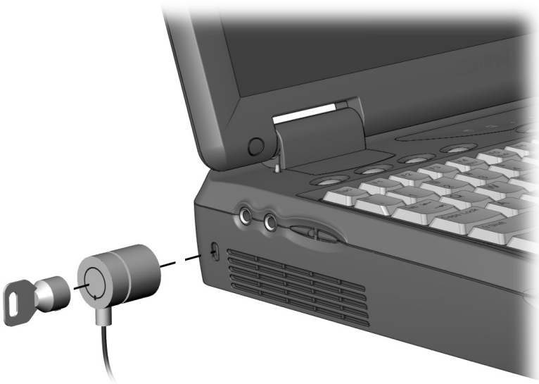
Attaching a Cable Lock Device
